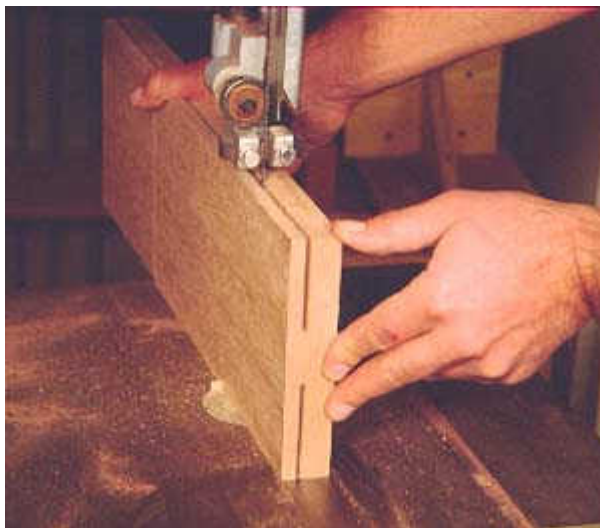
Photo 11- There is so little work for the band saw to do between the kerfs that you don't even need a fence to guide it, but using a fence will prevent wandering and leave a more consistent product, easier to deal with you are going to hand plane it smooth.
