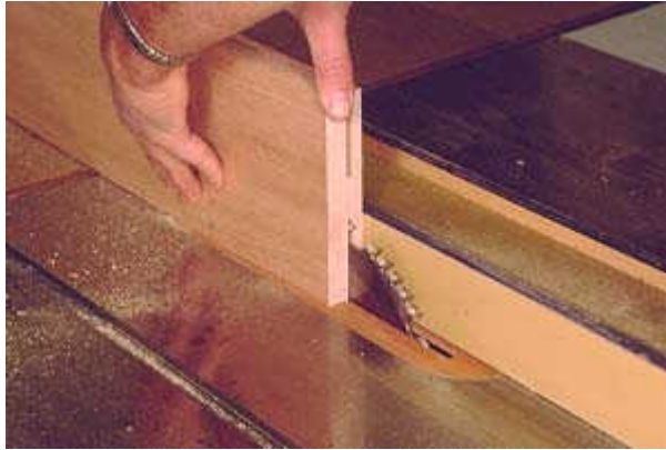
Photo 10- Even if your stock is so wide that the table saw can't complete the cut; use it to do most of the work so your band saw doesn't have to.
