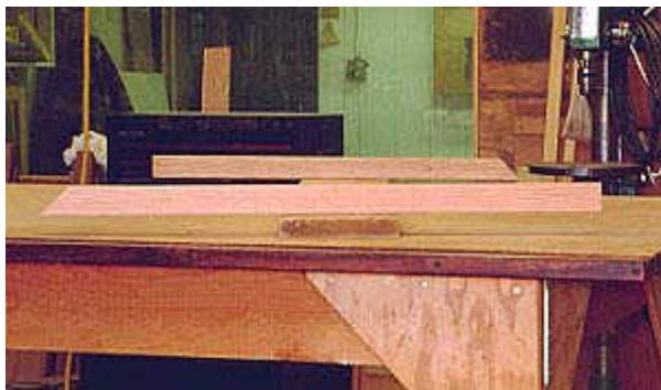
Photo 3- Winding sticks on a board that is almost flat. Note that the sticks are very close to being parallel to each other.
