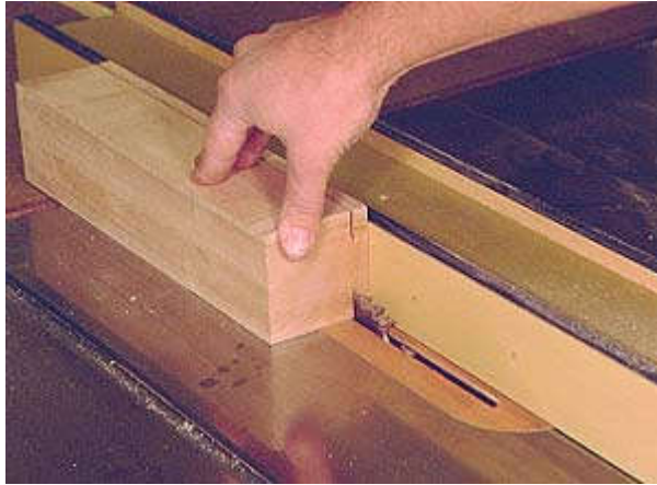
Photo 1- Resaw thick stock into thinner pieces at the table saw by making a progression of cuts. First make cuts at about an inch high as shown.
