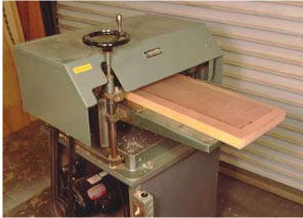
Photo 8- Plane very thin pieces by putting them on top of a thicker piece, in this case a section of a solid core door.
