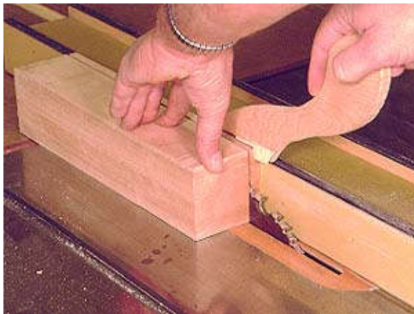
Photo 2- Raise the blade and make more cuts without moving the fence. When the thin part will be cut free, push it through with a push stick as shown.
