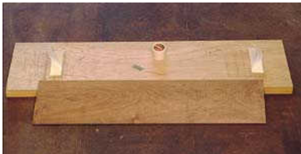
Photo 9- Double sided carpet tape is just the ticket to keep the thin stock down on the planing jig when you push it through the machine.
