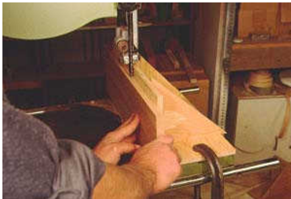
Photo 6- A long, or flat fence used for resaw. This fence does not allow you to adjust the direction of cut during the process. You must use test pieces to verify that the fence face is parallel to the cutting path. Ultimately this fence produces the most consistent result, if you start with straight stock.
