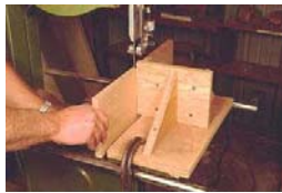
Photo 5- A point location fence used for resaw. This type of fence allows you to move the stock side to side as it is fed into the blade, adjusting the direction of cut while the cut is being made.
